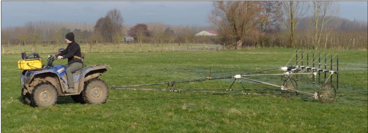
1. Advanced multi-channel magnetometer (fluxgate gradiometer) survey at the site of a 14th century castle (towed configuration with ATV).
