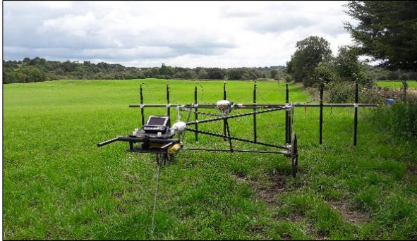
4. Advanced multi-channel magnetometer (fluxgate gradiometer) system (manual configuration).
